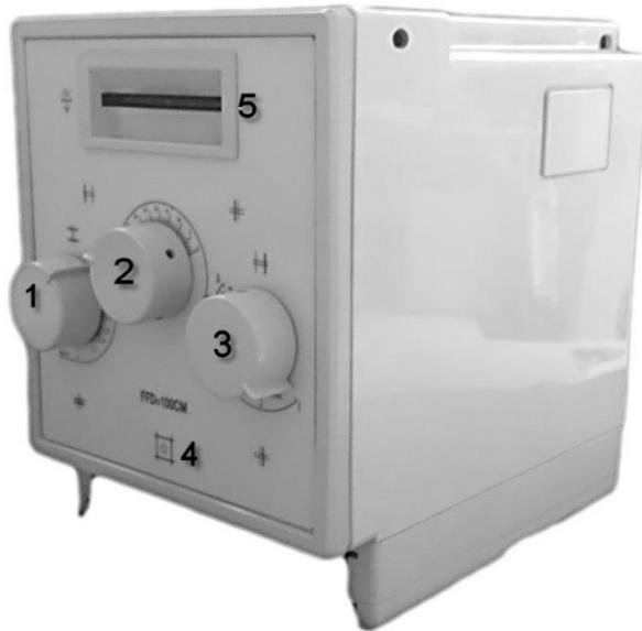
The collimator unit contains three control knobs, a push button and a filter.
